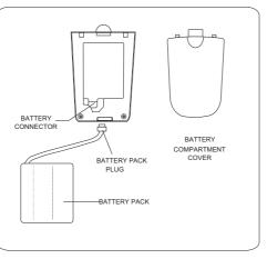
Remove the HANDSET BATTERY COMPARTMENT COVER by sliding it down.
